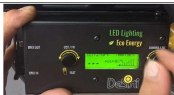
When the DISPLAY is in STAND BY Mode, please rotate KNOB 2 to act on the LIGHT INTENSITY Dimming. Clock Wise to increase the level and Counter Clock Wise to decrease it. Fine control:
