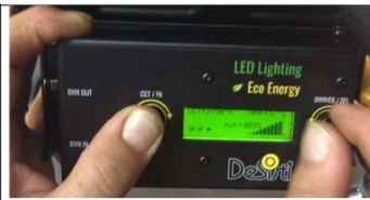
For faster Dimming Control keep KNOB 1 pressed and rotate KNOB 2: 1 full TURN of the KNOB 2 = 40% Dimming Variation
