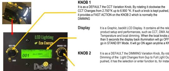
It is a Graphic, backlit LCD Display. It contains all the relevant information for the product setup and performances, such as CCT, DMX Address, DMX Level, LED . Temperature and local dimming. When the local knobs are not used for more than 5 seconds the display back illumination will go OFF and the display itself will
