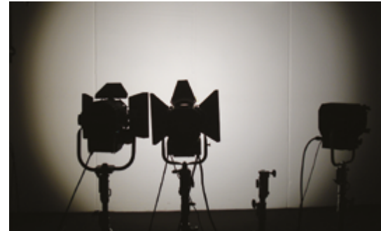
The light beam shown in full flood (60deg) has a even and flat field without any hot spots or drop off.
