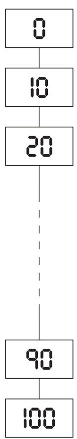
By pressing the enter button, the user will enter the quick dimmer menu: thanks to this menu it will be possible to increase and decrease the light intensity in steps of 10 (in a range from 0 to 100).
