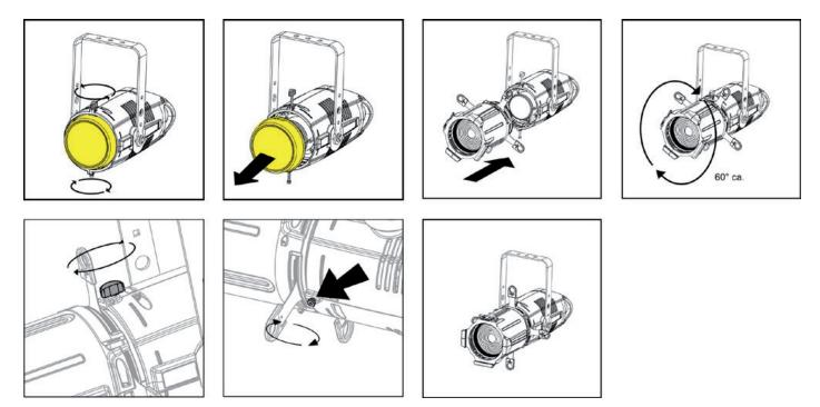
Remove the frontal cap by loosening the upper and lower screws enough to free the cap itself, set the optic's flange tilted about 60°. Insert the optic's flange into the body's receptacle and turn the optic 60° until it is firmly assembled to the projector body, free to rotate but not free to detach itself from the body. Ensure the optic to the body by tightening the two screws previously loosened.
